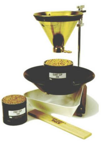
Fig. 1. A standard filling hopper and stand for the accurate filling of quart or pint cups for grain test weight determination.
