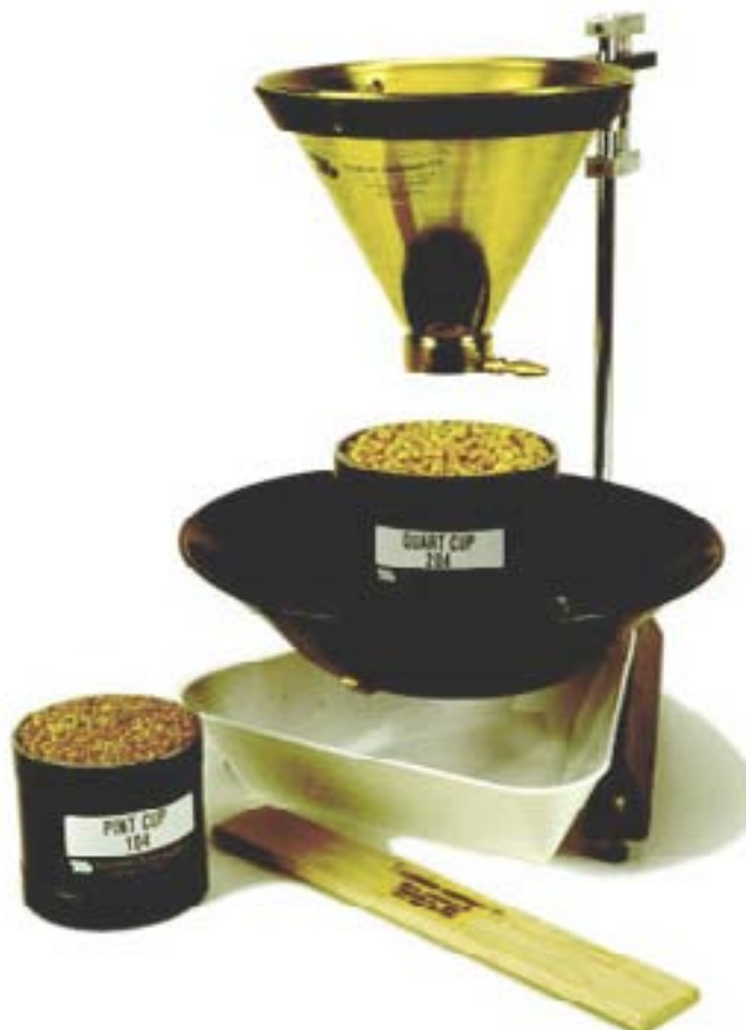
Figure 1. A standard filling hopper and stand for the accurate filling of quart or pint cups for grain test weight determination (Image: http://www.seedburo.com )
