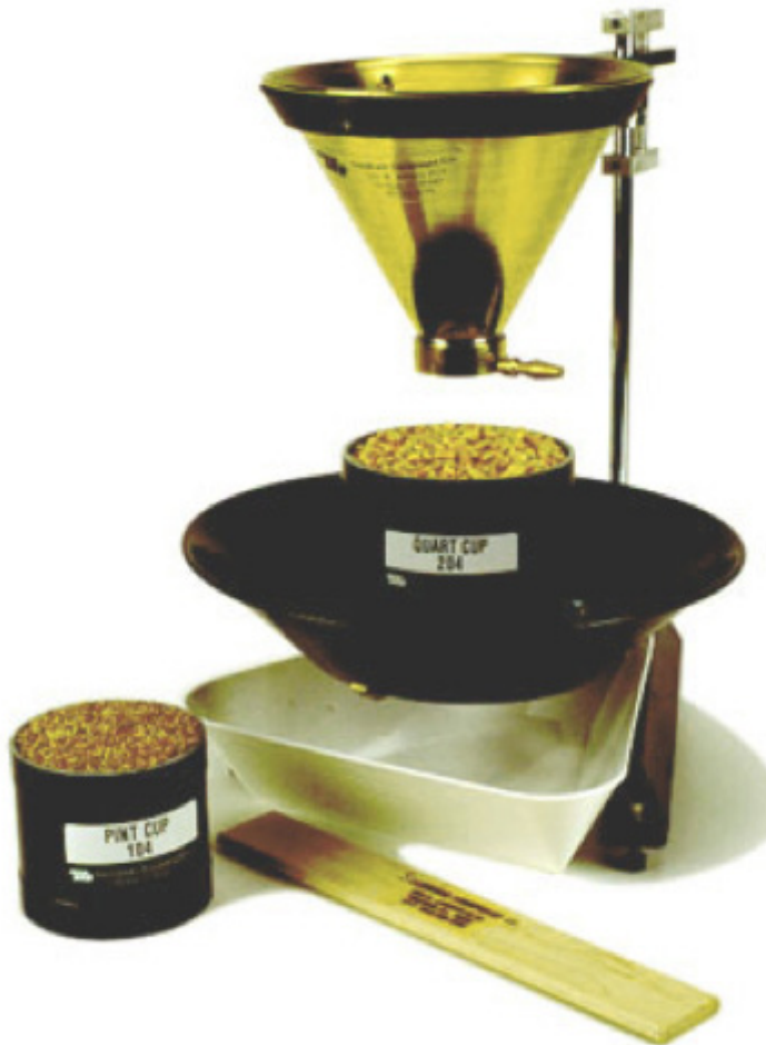
Figure 1. A standard filling hopper and stand for the accurate filling of quart or pint cups for grain test weight determination. (Image; www.seedbuero.com).
